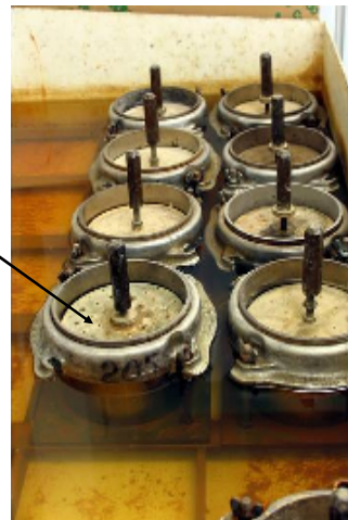
Soaking Samples for 4 days measure swelling and CBR
